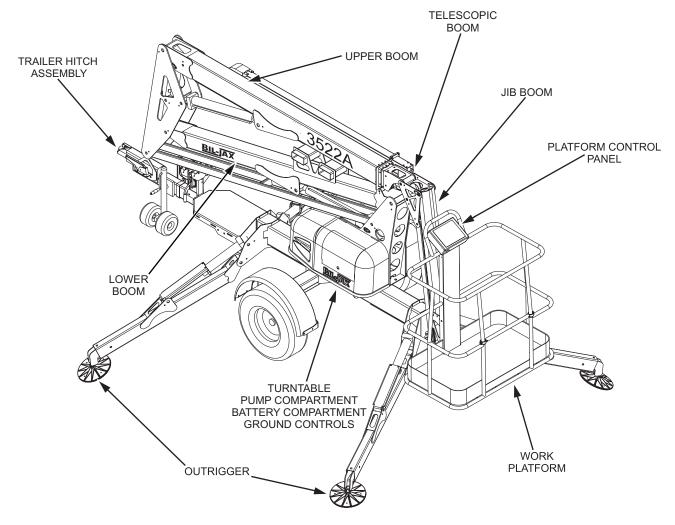
Figure 2-1. Model 3522A Articulating Boom Lift
